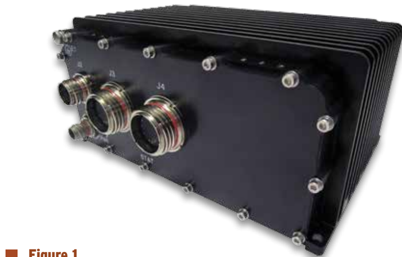
Figure 1 COBALT is a highly scalable embedded computer system, sealed and validated IP67, available with a wide selection of processor, storage, power and interface options.
